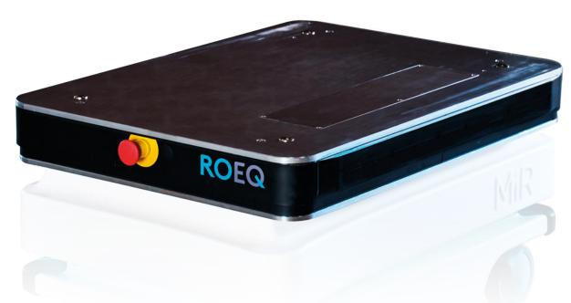
The TML150 is a lifter module for the MiR100, MiR200 and MiR250 + AM250. It enables the transport of trays and pallets. It can transport in raised position, reducing cycle time. You can mount the TML150 Forks on top to aid in picking up pallets and trays.
